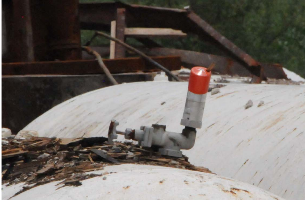
Figure 21. Anhydrous Ammonia Tank PRV, Post-Incident (Source: CSB)
