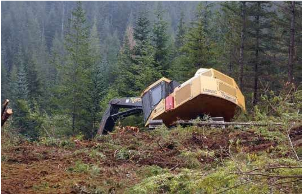
Feller-buncher/shovel logger tethered machine on steep slopes in Washington, United States of America © John J. Garland
