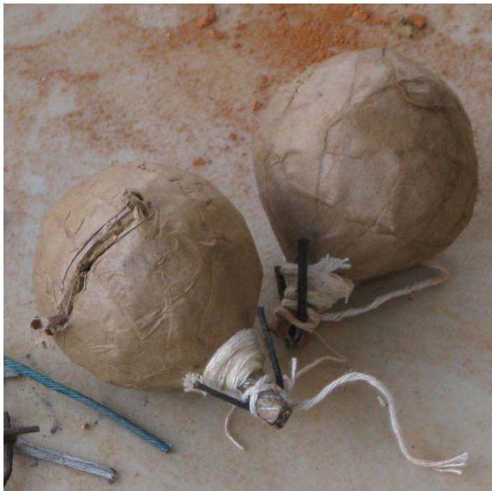
Figure 7. Slit aerial shell from DEI's first destruction
