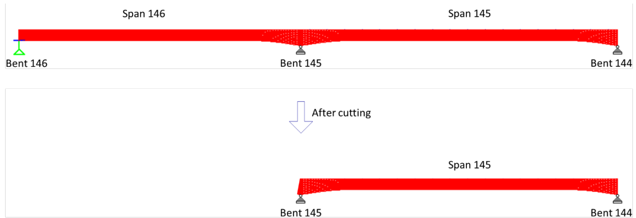
Figure 36 – Plate girders before and after cutting
