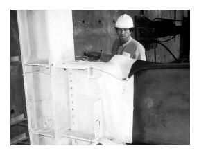
Engineers expect steel to be ductile, capable of extensive bending and deformation without fracturing, as shown in this test specimen. The development of cracks in the steel at relatively low levels of loading was unexpected.
