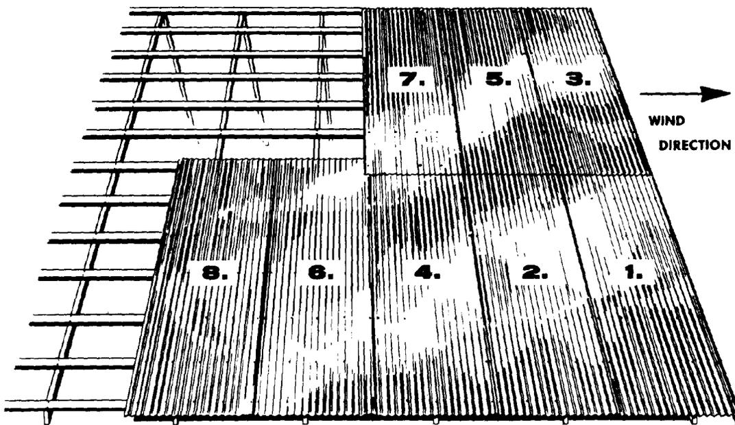
NOTE: PROVIDE A LIBERAL CALKING BEAD BETWEEN EACH END AND SIDE LAP OF SHEETS AND ACCESSORIES
