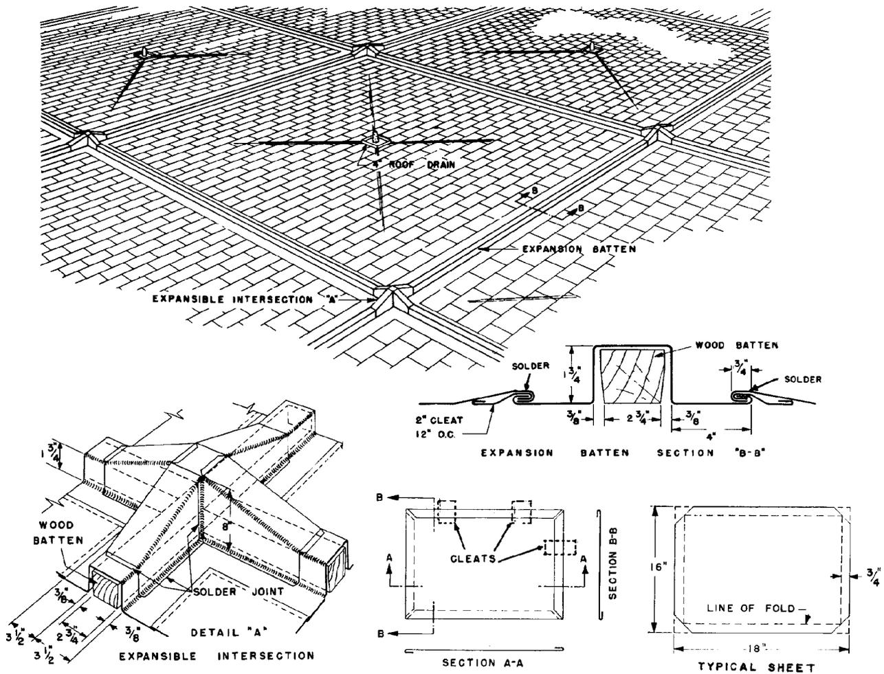
Figure 45. Flat seam roofing.
