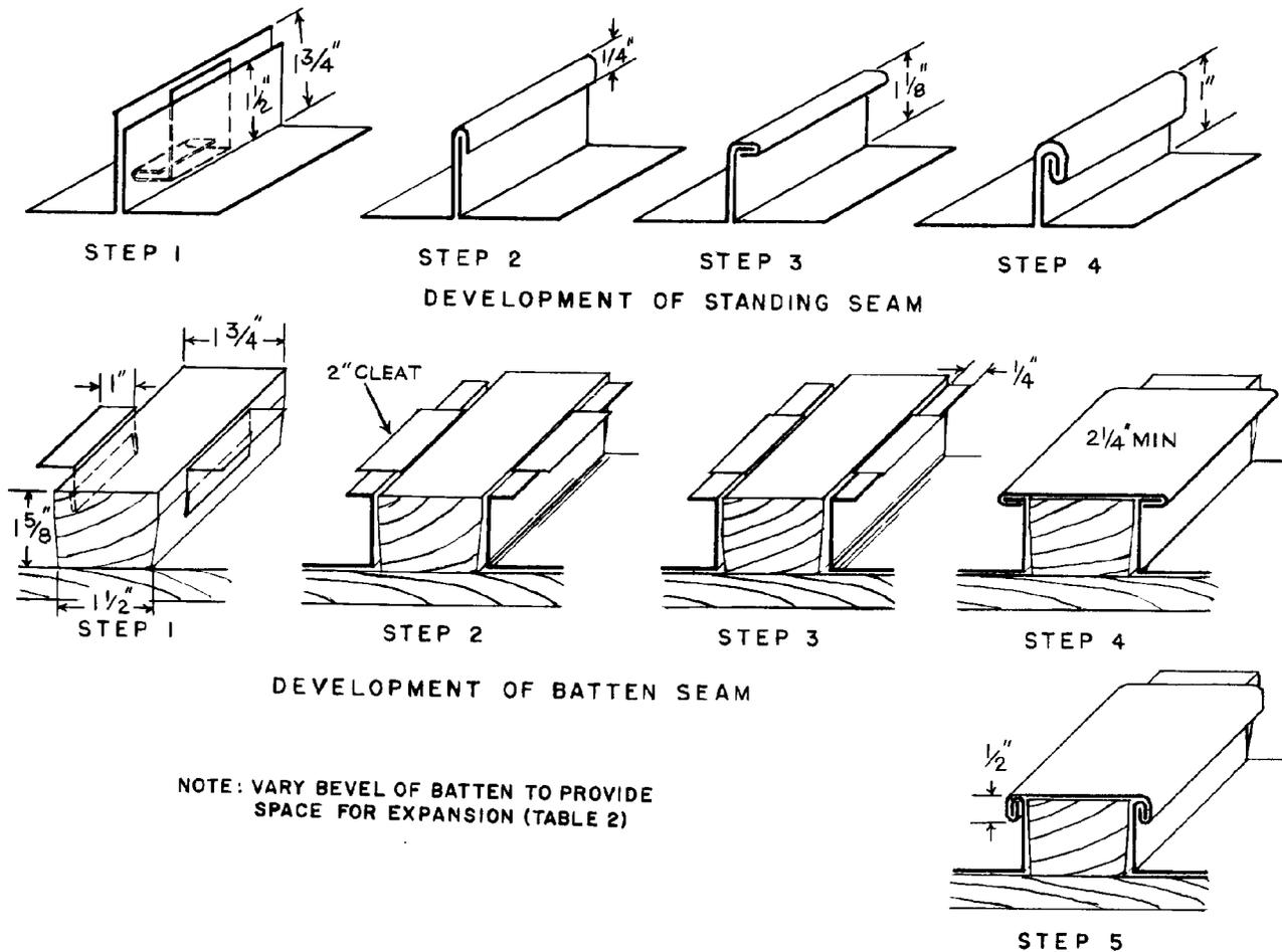
Figure 40. Development of standing and batten seams.
